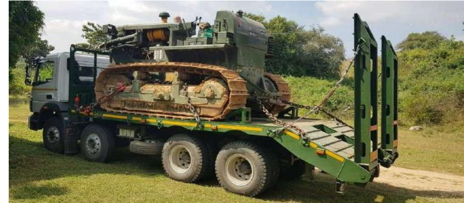
Flat Bed Truck (Loading Platform Dozer Weight of 20 Ton)
